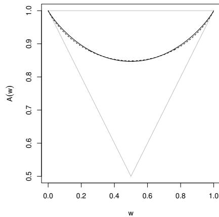
Fitted Pickands functions for the logistic (solid), Hüsler–Reiss (dots) and negative logistic (dashed) models. They are essentially identical.
