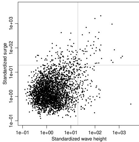
Simultaneous values of wave and surge height, transformed to unit Fréchet scale, with regions  $\mathcal{E}_{00}^*, \dots, \mathcal{E}_{11}^*$  determined by the grey lines marking the marginal 0.95 quantiles.
