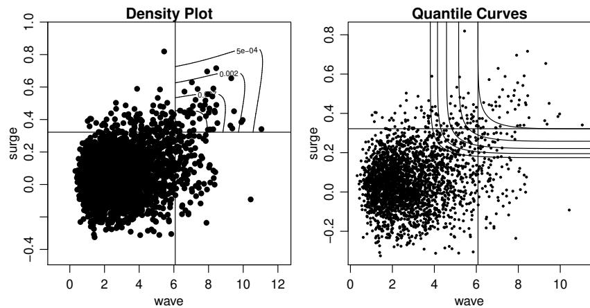
Diagnostic plots (from `plot(fit)`) for threshold fit to oceanographic data. (A bug prevents the points on the left from being smaller.) According to the help, the quantiles are at 0.75, 0.8, ..., 0.95 by default.
